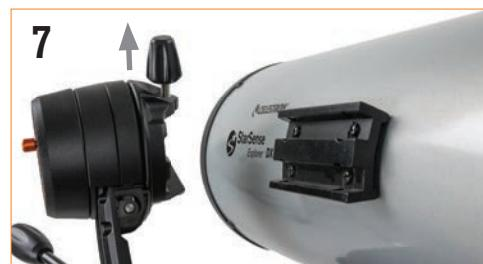
Turn the clamp assembly so that the locking screw is on top of the dovetail clamp. Hold the telescope tube next to the mount with the dovetail bar on the tube facing the clamp on the top of the mount arm.
