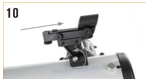
Slide the finderscope bracket into the dovetail slot on the telescope tube near the focuser. The large window on the finder should be facing the front of the telescope. Secure the bracket by tightening the setscrew on the dovetail slot.
