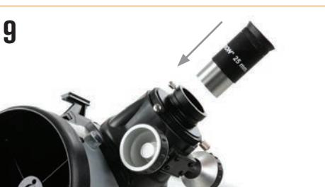
Remove the cap from the focuser and insert the barrel of the 25 mm eyepiece into the focuser. Tighten the setscrew to secure the eyepiece in place.
